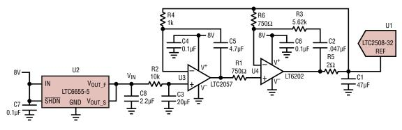
Figure 1. Filtered LTC6655 Output Increases SNR of LTC2508-32 32-Bit ADC by 6dB
